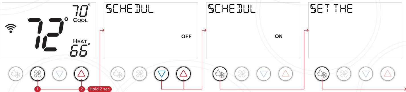
**Press and hold the fan and warmer (up) buttons for 2 seconds to enter schedule mode for programming a schedule.** While in schedule mode, press the mode button to advance through each setting for each day of the week and each time period of each day.
