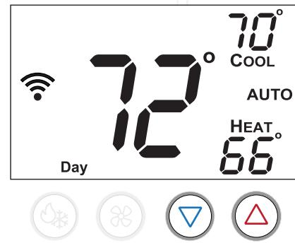
**When the schedule is enabled,** the warmer (up) and cooler (down) buttons raise and lower the setpoints as usual. Adjustments made this way remain in place until the next schedule event is reached.
