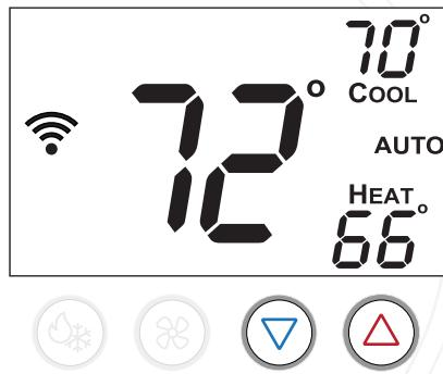
**When set to auto mode,** pressing the warmer (Up) up arrow button increases both the heat and cool setpoints. Pressing the cooler (down) arrow button decreases both the heat and cool setpoints.
