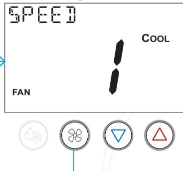
Press the warmer (up) and cooler (down) buttons to cycle through the available fan speeds of auto and 1 (low) through 5 (high).
