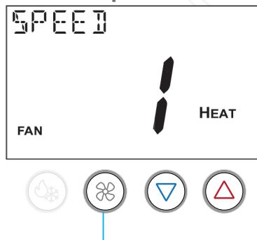
Press the warmer (up) and cooler (down) buttons to cycle through available fan speeds of auto and 1 (low) through 5 (high).
