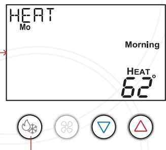
Press the warmer (up) or cooler (down) buttons to adjust the heat setpoint for the morning schedule event. Press the mode button to advance to the next step.
