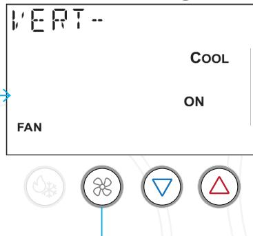
Press the warmer (up) and cooler (down) buttons to toggle the cool mode vertical swing off and on.
