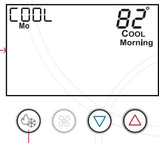
Press the warmer (up) or cooler (down) buttons to adjust the cool setpoint for the morning schedule event. Press the mode button to advance to the next step.
