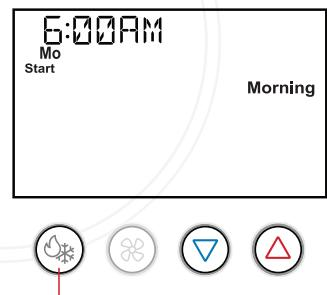
Press the warmer (up) or cooler (down) buttons to adjust the morning schedule event start time in 15 minute increments. The day of the week being scheduled appears below the time selection, and the name of the schedule event ("morning" in this case) also appears on the screen. Press the mode button to advance to the next step.
