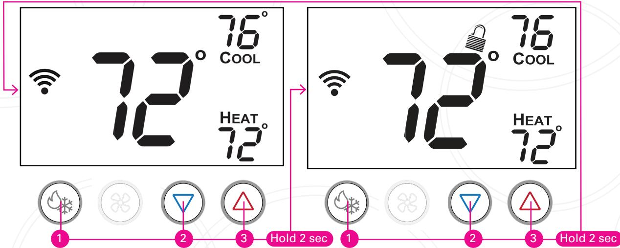
**To disable, or “lock” the keypad,** press the warmer (up) and cooler (down) buttons and hold for two seconds. When the lock icon appears on the display, release the buttons.
