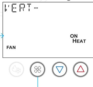
Press the warmer (up) and cooler (down) buttons to toggle the heat mode vertical swing off and on.
