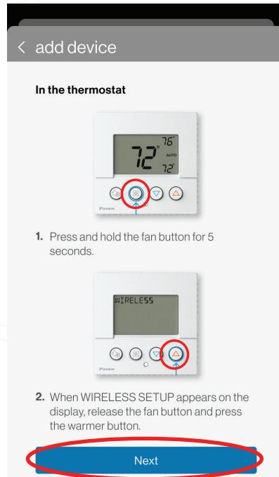
1. After your Daikin **ONE Lite** thermostat is connected to Wi-Fi, select "Next". (If not starting on this screen, select "Add Device", then select "Daikin ONE lite connected thermostat" and a location, and press "Next".)
