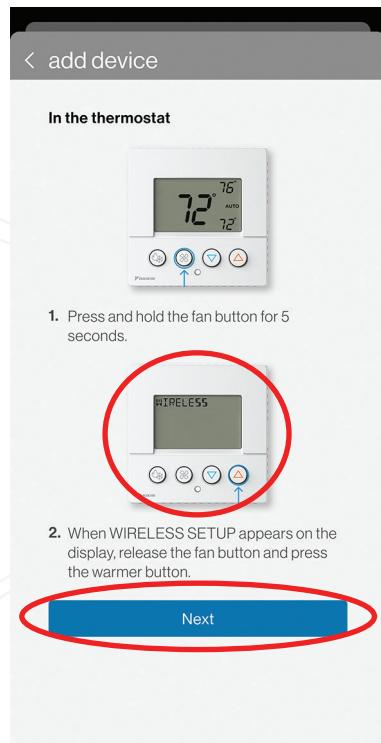
4. Press the fan button for 5 seconds to put the thermostat in "WIRELESS SETUP", then select "Continue".
