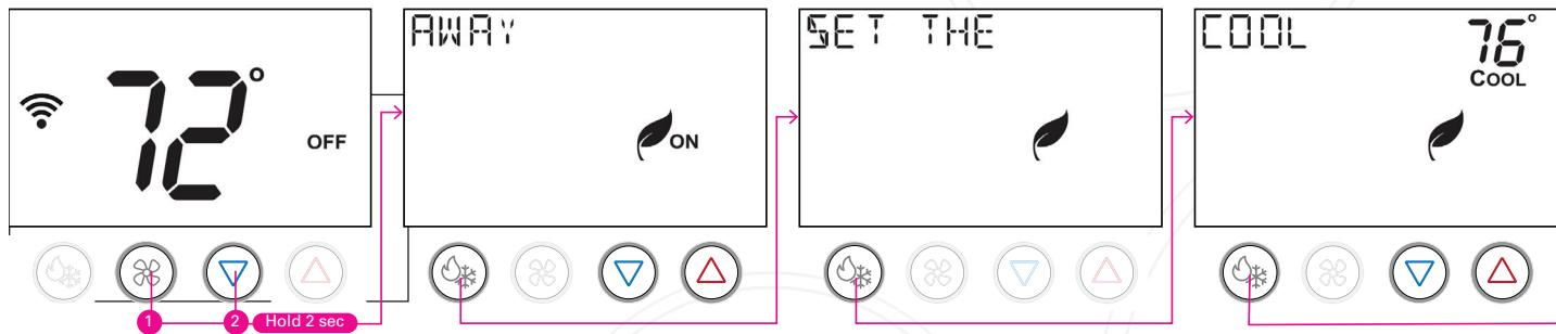
**Press and hold the fan and cooler (down) buttons** to enter the settings for Away mode.
