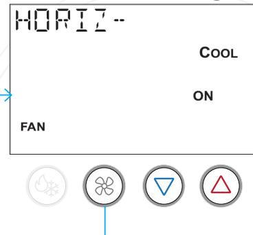
Press the warmer (up) and cooler (down) buttons to toggle the cool mode horizontal swing off and on.
