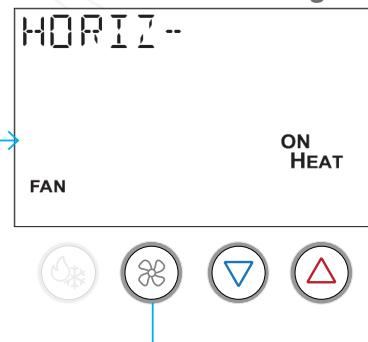
Press the warmer (up) and cooler (down) buttons to toggle the heat mode horizontal swing off and on.
