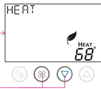
**Press the warmer (up) and cooler (down) buttons** to adjust the heating setpoint.
